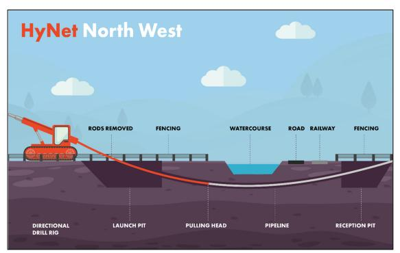
Insert 3.4 - Illustration of HDD Technique
