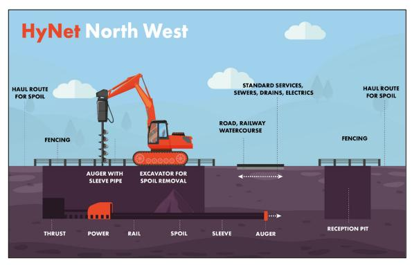
Insert 3.5 - Illustration of Auger Bore Technique
